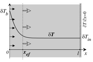
Fig. 1. Configuration of the piston effect in a layer.
